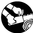
**To reduce the risk of accidents and injuries, always hold your saw firmly with both hands:** Right hand on the control handle, even if you are left-handed. To ensure safe control, wrap your fingers tightly around both handles.
